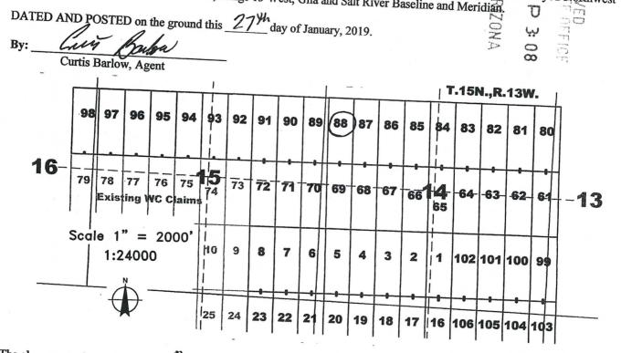
The above map depicts the WC  $\_$ \_\_ lode mining claim, which is located in Section(s)\_\_\_\_/4/\_\_\_, Township 15 North, Range 13 West, Gila and Salt River Baseline and Meridian, Mohave County, Arizona. The claim corners, end centers, and location monuments are marked by 2 inch by 2 inch by 5 foot wooden posts with aluminum tags. The bearings and distances between claims are as depicted on the map and tied as noted above.
