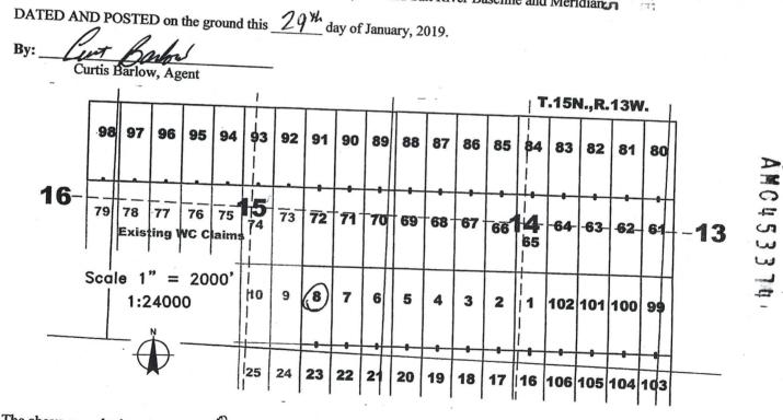
The above map depicts the WC  $\_$  B lode mining claim, which is located in Section(s)  $\_$  5 5 5 5 5 5 5 5 15 North, Range 13 West, Gila and Salt River Baseline and Meridian, Mohave County, Arizona. The claim corners, end centers, and location monuments are marked by 2 inch by 2 inch by 5 foot wooden posts with aluminum tags. The bearings and distances between claims are as depicted on the map and tied as noted above.
