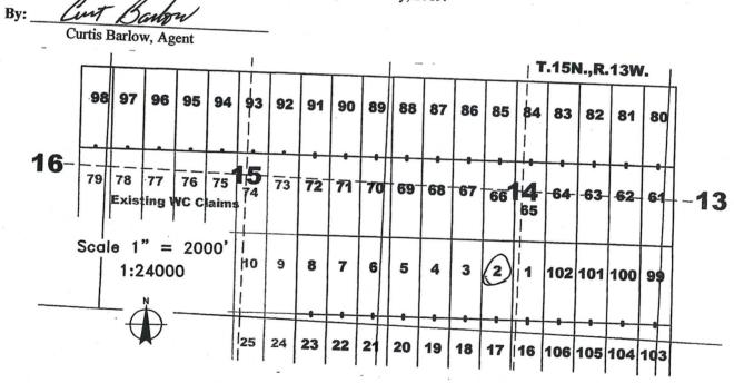
The above map depicts the WC 2 \_\_ lode mining claim, which is located in Section(s)\_\_\_\_\_\_ North, Range 13 West, Gila and Salt River Baseline and Meridian, Mohave County, Arizona. The claim corners, end centers, and location monuments are marked by 2 inch by 2 inch by 5 foot wooden posts with aluminum tags. The bearings and distances between claims are as depicted on the map and tied as noted above.
