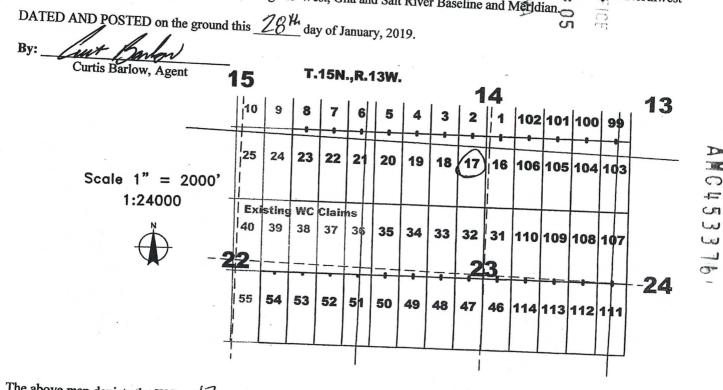
The above map depicts the WC \_\_\_\_\_ lode mining claim, which is located in Section(s) \_\_\_\_\_ 14, 23 \_\_\_\_, Township 15 North, Range 13 West, Gila and Salt River Baseline and Meridian, Mohave County, Arizona. The claim corners, end centers, and location monuments are marked by 2 inch by 2 inch by 5 foot wooden posts with aluminum tags. The bearings and distances between claims are as depicted on the map and tied as noted above.
