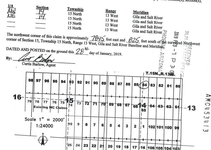
The above map depicts the WC  $\underline{\beta}$ lode mining claim, which is located in Section(s)\_ North, Range 13 West, Gila and Salt River Baseline and Meridian, Mohave County, Arizona. The claim corners, end centers, and location monuments are marked by 2 inch by 2 inch by 5 foot wooden posts with aluminum tags. The bearings and distances between claims are as depicted on the map and tied as noted above.
