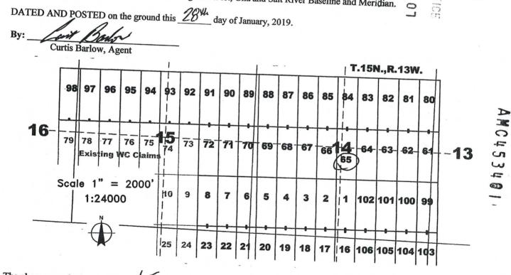
The above map depicts the WC 65 lode mining claim, which is located in Section(s) North, Range 13 West, Gila and Salt River Baseline and Meridian, Mohave County, Arizona. The claim corners, end centers, and location monuments are marked by 2 inch by 2 inch by 5 foot wooden posts with aluminum tags. The bearings and distances between claims are as depicted on the map and tied as noted above.
