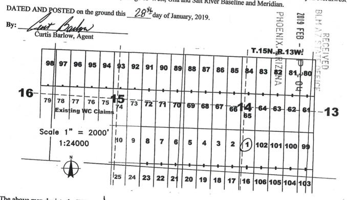
The above map depicts the WC lode mining claim, which is located in Section(s) North, Range 13 West, Gila and Salt River Baseline and Meridian, Mohave County, Arizona. The claim corners, end centers, and location monuments are marked by 2 inch by 2 inch by 5 foot wooden posts with aluminum tags. The bearings and distances between claims are as depicted on the map and tied as noted above.
