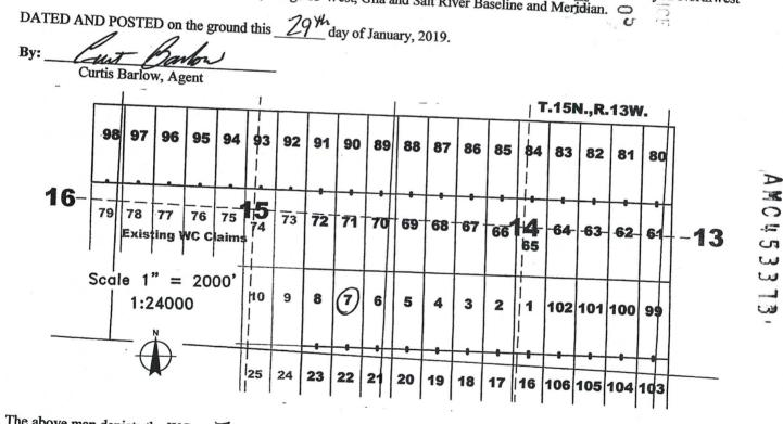
The above map depicts the WC \_\_ lode mining claim, which is located in Section(s)\_\_\_\_\_\_, Township 15 North, Range 13 West, Gila and Salt River Baseline and Meridian, Mohave County, Arizona. The claim corners, end centers, 7 and location monuments are marked by 2 inch by 2 inch by 5 foot wooden posts with aluminum tags. The bearings and distances between claims are as depicted on the map and tied as noted above.
