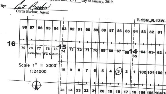
The above map depicts the WC 3 lode mining claim, which is located in Section(s) North, Range 13 West, Gila and Salt River Baseline and Meridian, Mohave County, Arizona. The claim corners, end centers, and location monuments are marked by 2 inch by 2 inch by 5 foot wooden posts with aluminum tags. The bearings and distances between claims are as depicted on the map and tied as noted above.
