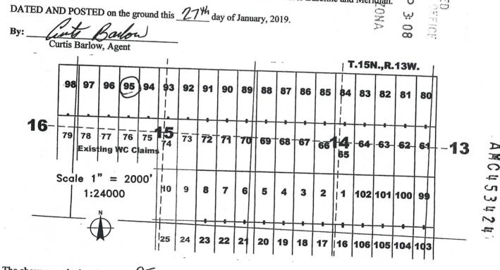
The above map depicts the WC \_\_\_\_\_\_ lode mining claim, which is located in Section(s)\_\_\_\_\_ North, Range 13 West, Gila and Salt River Baseline and Meridian, Mohave County, Arizona. The claim corners, end centers, and location monuments are marked by 2 inch by 2 inch by 5 foot wooden posts with aluminum tags. The bearings and distances between claims are as depicted on the map and tied as noted above.
