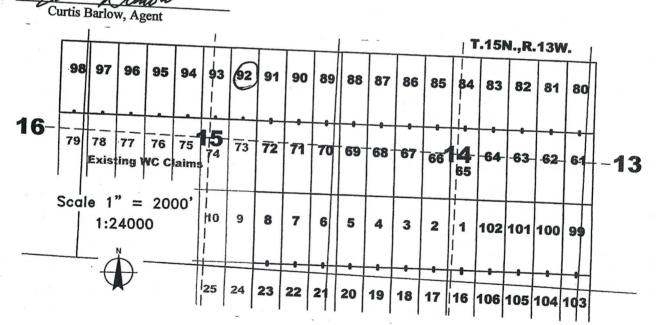
The above map depicts the WC 92 lode mining claim, which is located in Section(s) North, Range 13 West, Gila and Salt River Baseline and Meridian, Mohave County, Arizona. The claim corners, end centers, and location monuments are marked by 2 inch by 2 inch by 5 foot wooden posts with aluminum tags. The bearings and distances between claims are as depicted on the map and tied as noted above.
