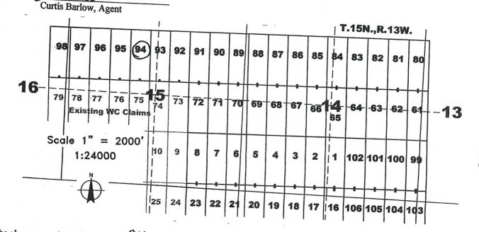
The above map depicts the WC  $_{99}$ \_\_\_ lode mining claim, which is located in Section(s)\_\_\_\_ North, Range 13 West, Gila and Salt River Baseline and Meridian, Mohave County, Arizona. The claim corners, end centers, \_\_\_\_, Township 15 and location monuments are marked by 2 inch by 2 inch by 5 foot wooden posts with aluminum tags. The bearings and distances between claims are as depicted on the map and tied as noted above.
